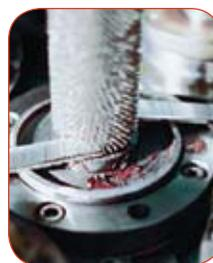
At left: The patented Spine Fin™ machine wraps aluminum spined ribbon tightly onto adhesive coated tubing. At right: The colored adhesive has extruded out from under the fins, locking them together and sealing out moisture.
